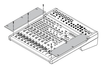
3. Mount the unit into the rack, and fasten it into place.
