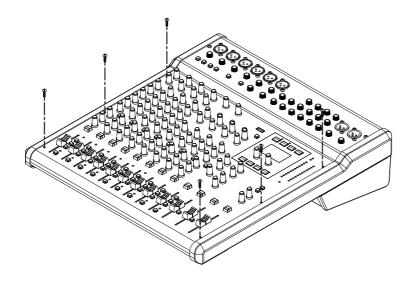
2. Use the screws of the accessories install the rack-mount kit on the mixer
